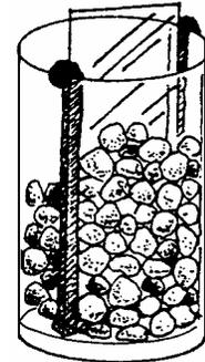
Place a strip of putty or silicone against the inner sides and bottom of a clear glass beaker (see illustration). Measure the diameter of the beaker and cut a piece of acetate to fit snugly in the center of the beaker. Insert the acetate into the putty strip inside the beaker so that two separate compartments are formed. (The acetate represents a relatively impermeable dike inside the shield volcano.) Gently add lava rocks to both sides of the beaker.
